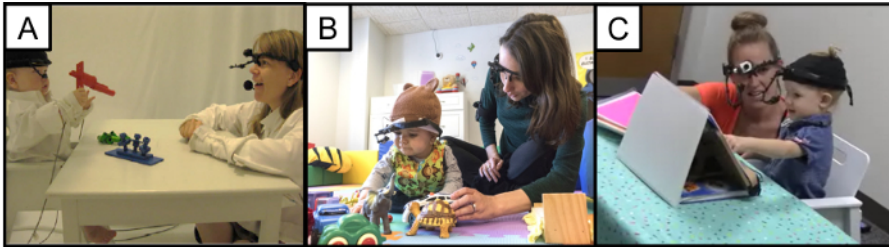
Figure 1. Head-mounted eye tracking employed in three different contexts: (A) tabletop toy play, (B) toy play on the floor, and (C) reading a picture book. Please click here to view a larger version of this figure.
