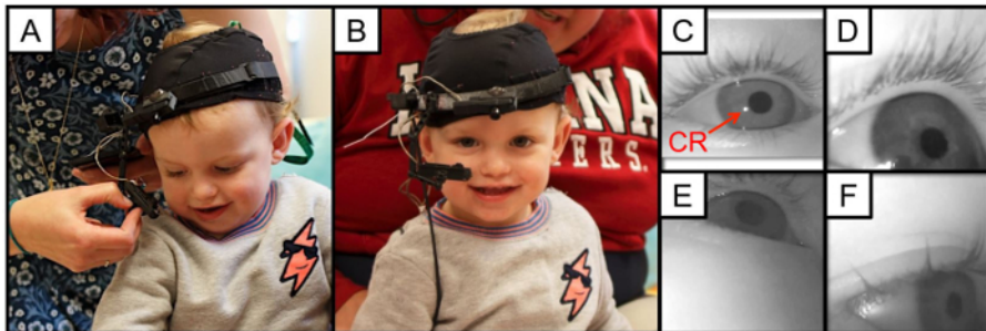
Figure 2. Setting up the head-mounted eye-tracking system. (A) A researcher positioning an eye tracker on an infant. (B) A well-positioned eye tracker on an infant. (C) Good eye image with large centered pupil and clear corneal reflection (CR). (D, E, F) Examples of bad eye images. Please click here to view a larger version of this figure.
